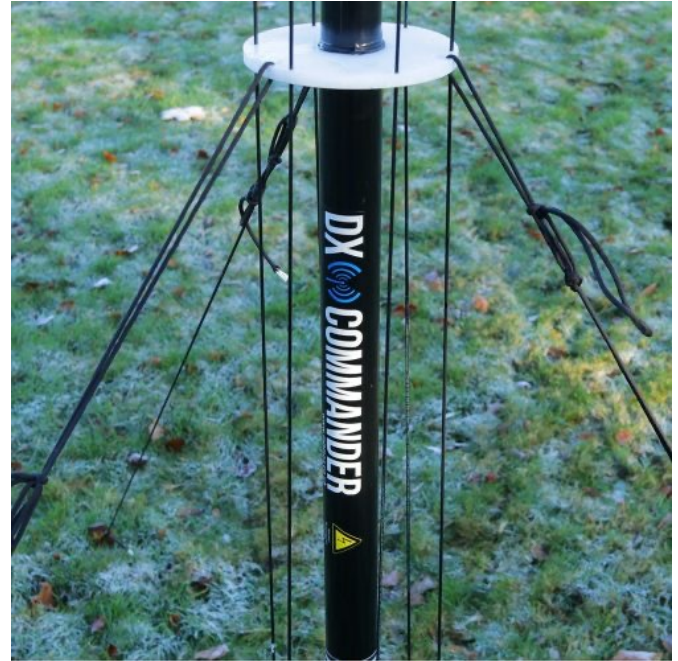
Figure 1. Detail of the wire guide/guy ring on a DX Commander vertical.
