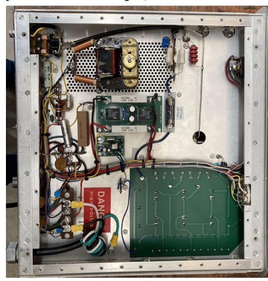
parasitic oscillation at 200-400 MHz especially when operating on 15 and 10m, which isn't too unusual for this amplifier. Careful tuning. especially keeping the loading a bit high, pretty well can avoid this. There's lots of reasons behind all this... Suffice it to say Heathkit that made certain economical decisions. Anyway, Greg now has another classic amp to add to his boat anchor station.
