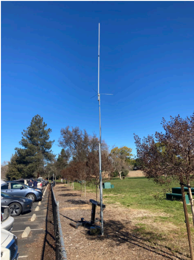
KQ6DI's portable digipeater & antenna at Independence Park
